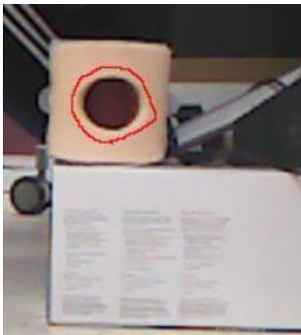
Figure 5: The drawing contour of wound model. The red contour is drawn on the color image with a mouse.
